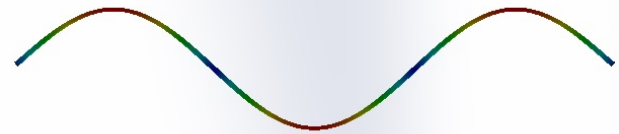
Figure 10. Elastic rotor third normal mode for selected input data (simply supported)
