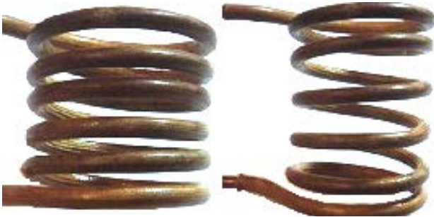
Figure 6. Experimental inductors developed through models presented at figures 3 and 4.
