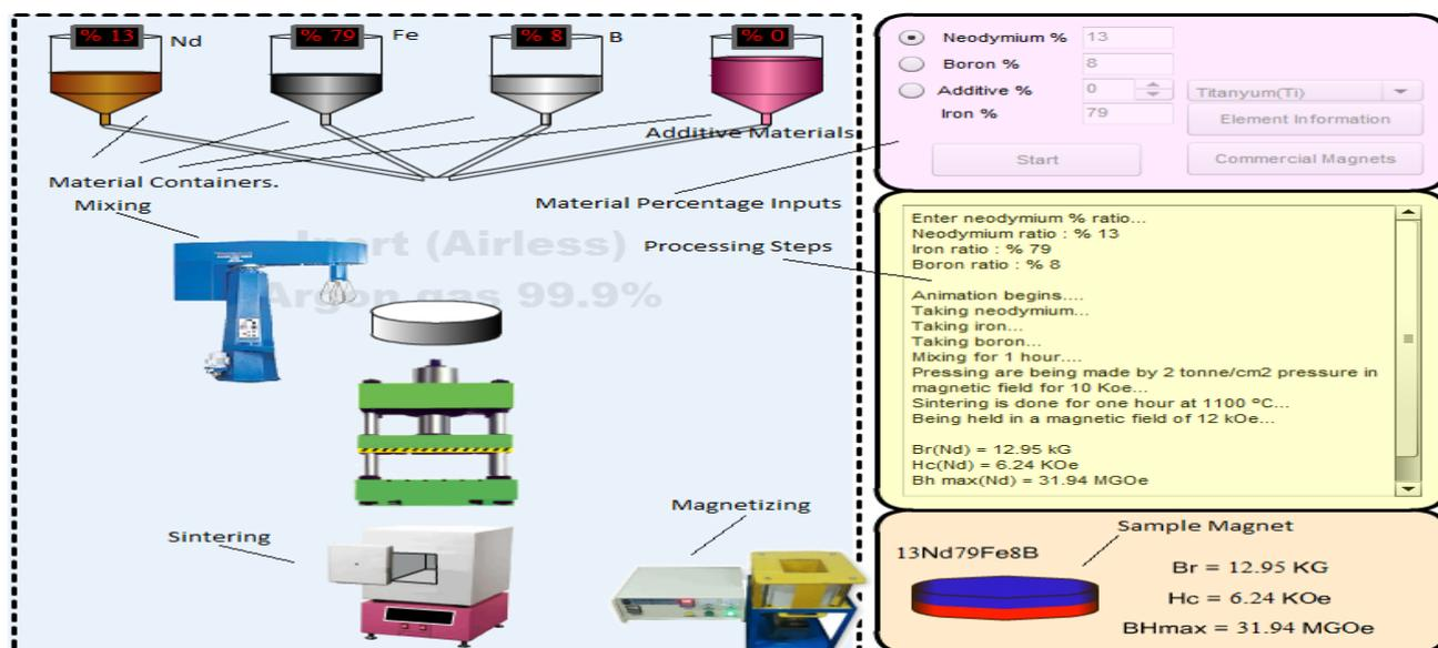
Figure 2. Screen shot of the developed virtual laboratory software.
