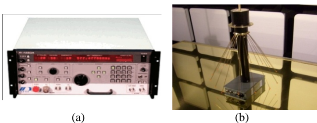
Figure 2. TEMPEST receiver (a) and wideband antenna (b) [18].
