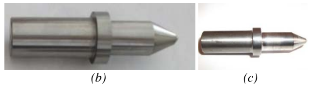
Figure 2: Friction drilling tool key dimensions (a), HSS tool image (b), and WC tool image (c)
