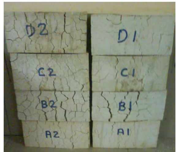
Figure 8. A group of samples held in oven at 900 °C
