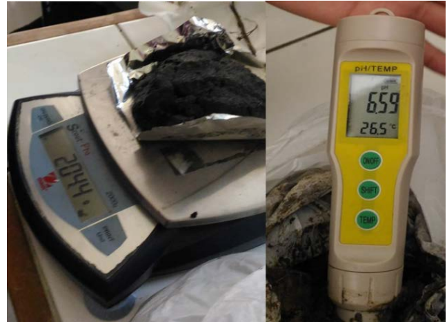
Figure 2. pH measurement, electrical conductivity of soil samples.
