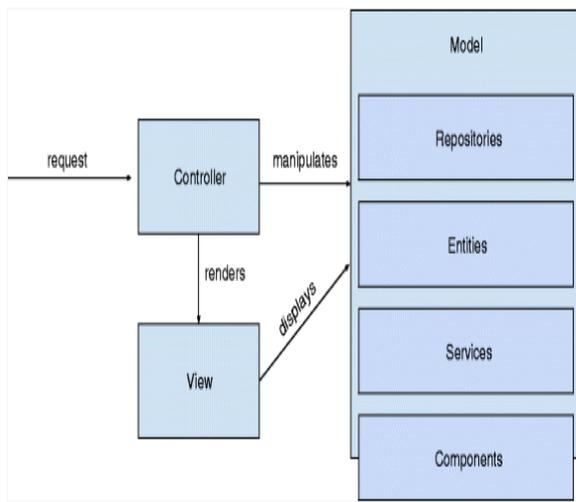
Figure 1. Model View Controller (MVC) [2].
