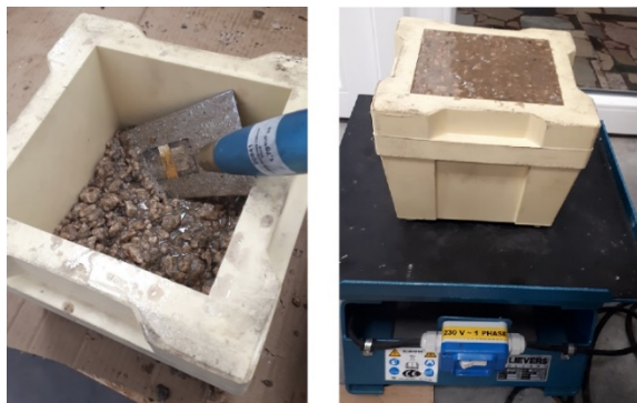
Figure 7. Filling the mold and vibration on Lievers LTT 40/40
