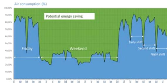
Figure 3. Demand profile in typical pneumatic system
