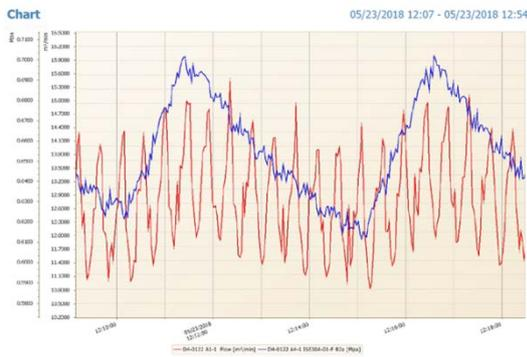
Figure 7. Results of the pressure and consumption measurement of a production line
