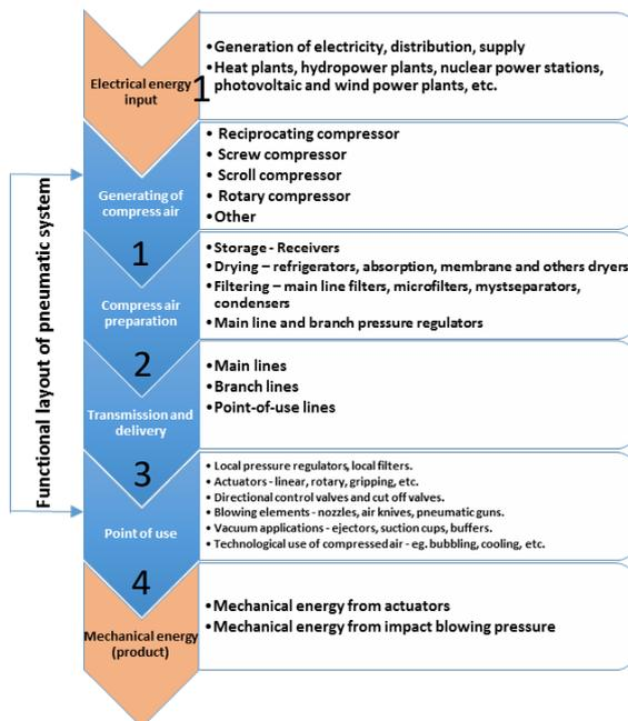
Figure 1. Energy flows in the compressed air system
