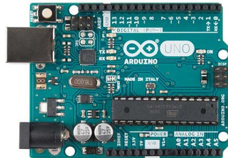
Figure 2. Microcontroller Arduino Uno
