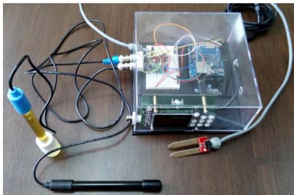
Figure 6. Wireless system for measuring pH, electrical conductivity and soil humidity
