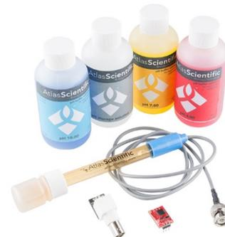
Figure 3. PH sensor and its calibration solutions
