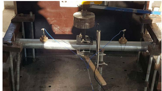
Figure 6. Measurement devices on test member
