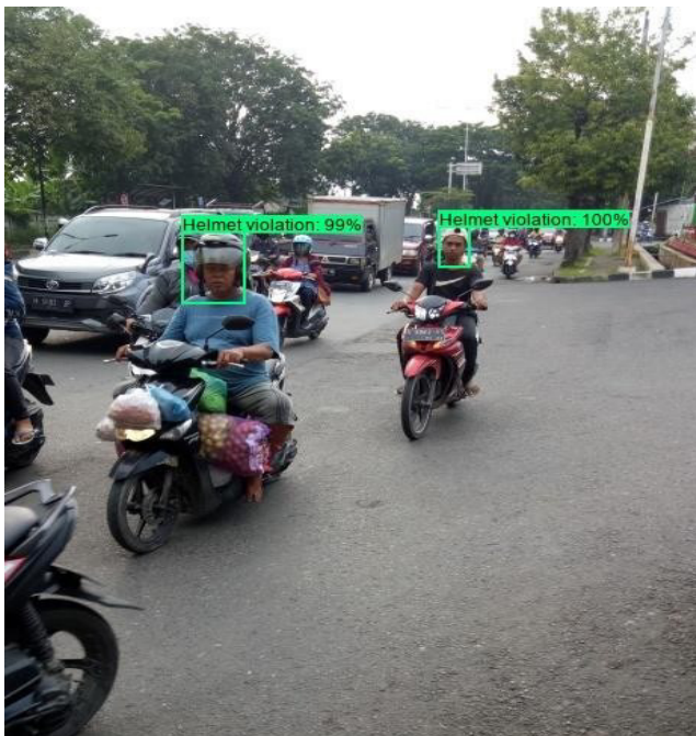
Figure 4. Helmet violation detection with false (left object) and correct (right object) detection results
