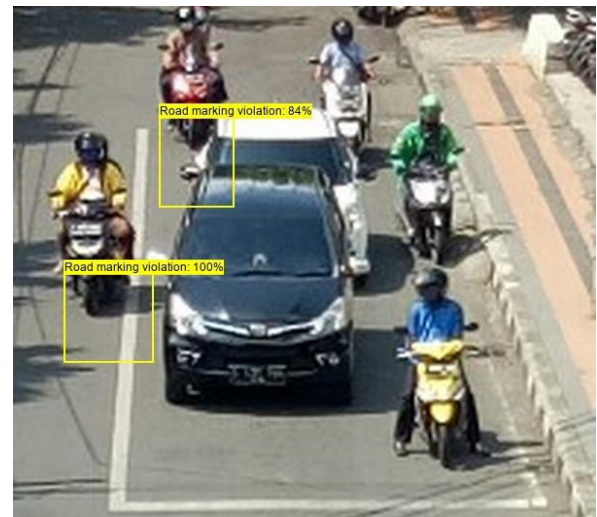
Figure 6. Mark violation detection with correct (left object) and false (right object) detection results
