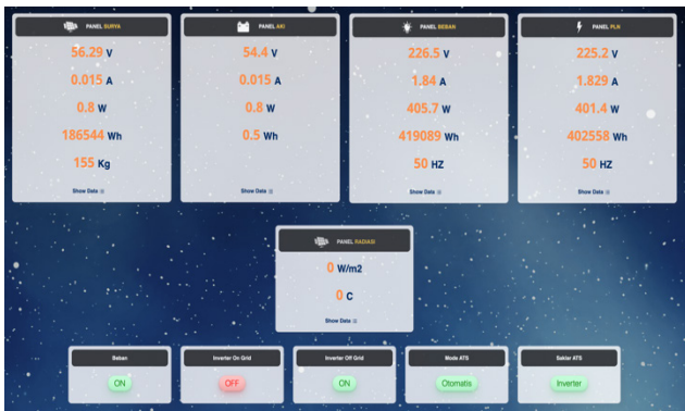
Figure 10. Solar PV system monitoring dashboard
