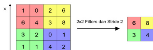
Figure 1. Pooling layer with 2x2 filter
