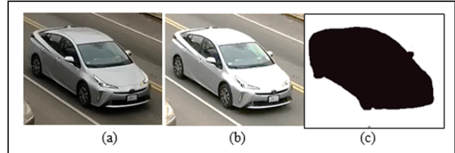
Figure 2. Preprocessing results (a) Original RGB image (b) Pre-processed image (c) subtracted background image
