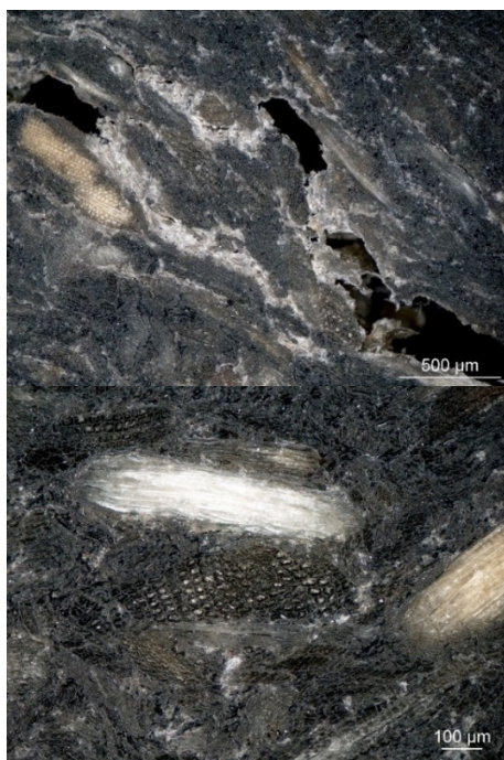
Figure 2. Interface High-density polyethylene (HDPE) matrix and wood particle, avoids between wood particle and plastic matrix (WPC product) [9]
