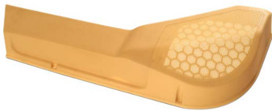
Figure 4. Part of car door made of wood plastic composite [11]
