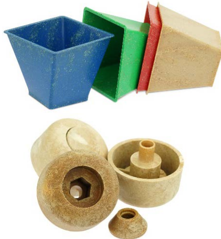
Figure 5. Compostable cups and furniture legs (company: JELUplast Germany, up: PLA matrix + 50 % wood fibre / down: PP matrix + 50 % wood fibre) [12]
