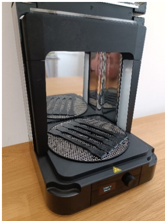
Figure 2. Irradiation chamber with testing specimens
