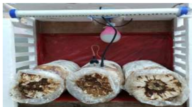
Figure 7. Baglog container with automatic control over water pH, temperature, and humidity of Baglog by developed hardware and software systems
