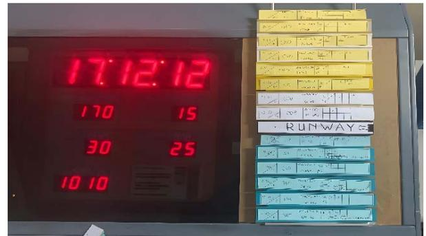
Figure 8. Manual flight strip
