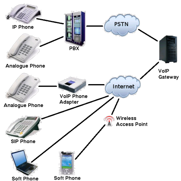
Figure 1. System configuration of the telephone exchange [10]
