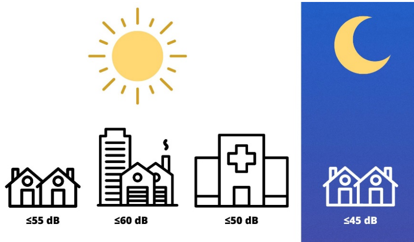
Figure 6. Permissible limit values for environmental noise
