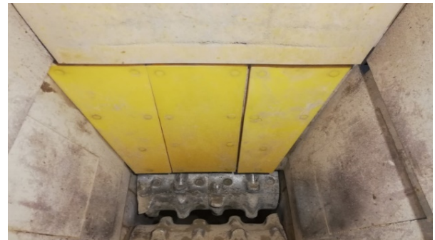
Figure 3. Noise reduction in front wall of the hopper on the roller crusher
