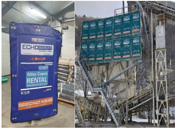
Figure 4. Mobile Echo Barrier and its location at the sorter
