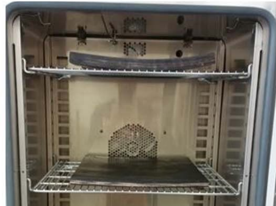
Figure 7. Conveyor belt specimens placed inside the Heratherm oven
