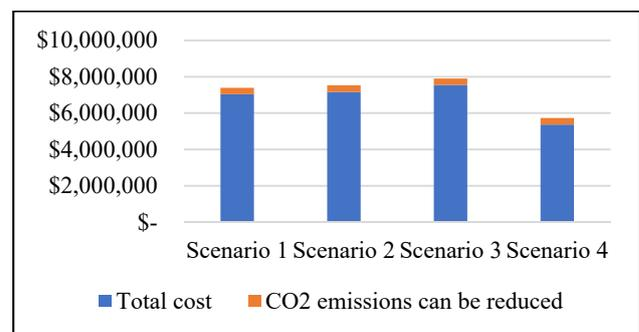
Figure 8. CO<sub>2</sub> emissions that can be reduced compared with the total cost of the solar PV system in the Bekasi case study
