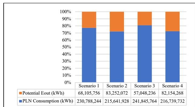
Figure 5. Potential energy output solar PV system compared with PLN electricity consumption at Semarang case study
