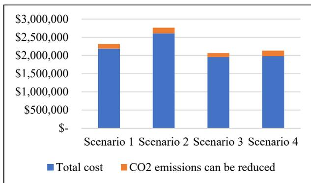
Figure 9. CO<sub>2</sub> emissions that can be reduced compared with the total cost of the solar PV system in the Semarang case study
