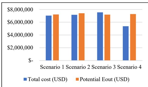
Figure 6. Potential energy output compared with the total cost of the solar PV system at the Bekasi case study
