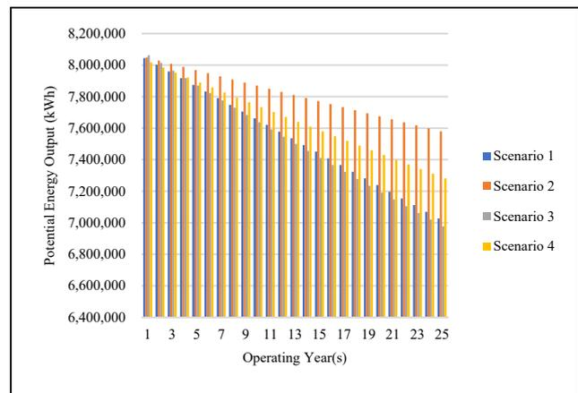
Figure 2. Potential electrical energy output (kWh) of Semarang case study solar rooftop PV system
