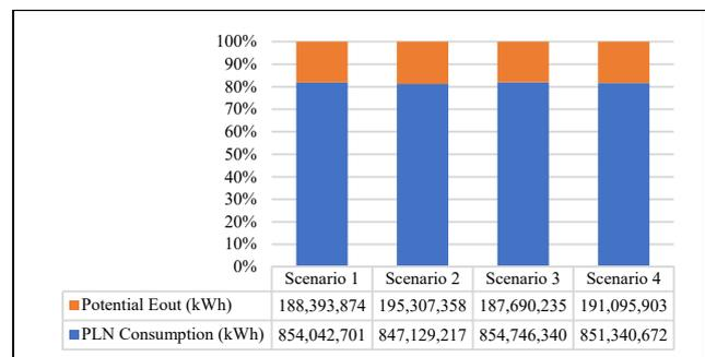
Figure 4. Potential energy output solar PV system compared with PLN electricity consumption at Bekasi case study
