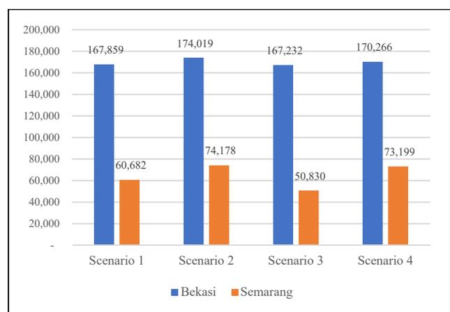
Figure 3. Potential electrical energy output (kWh) of Semarang case study solar rooftop PV system
