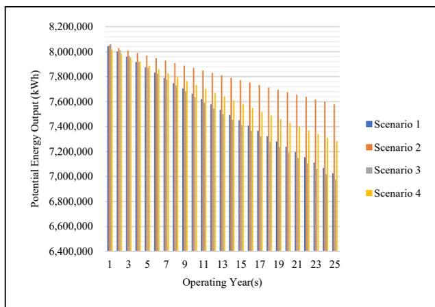
Figure 1. Potential electrical energy output (kWh) of Bekasi case study solar rooftop PV system
