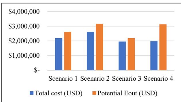
Figure 7. Potential energy output compared with the total cost of the solar PV system at the Semarang case study
