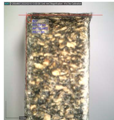
Figure 7. Sample 17 – principle of measured parameter r_k on the sample
