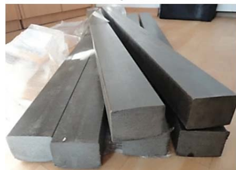
Figure 4. Extruded WPC profile for AWJ cutting, thickness of material 40 mm (author's archive)
