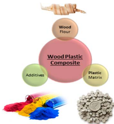
Figure 1. Components of Wood Plastic Composite (wood flour / plastic matrix – PP / PE / PVC, additives) [14-16]
