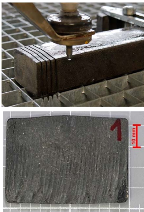
Figure 5. AWJ cutting of natural composite material (author's archive)
