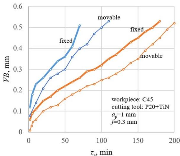
Figure 4. Flank wear of a fixed (thin line) and movable (bold line) turning tool (orange for cutting speed  $v_c=50$  m.min<sup>-1</sup> and blue for  $v_c=100$  m.min<sup>-1</sup>)
