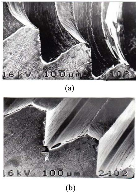
Figure 10. Thread profile formed by (a) classical and (b) ultrasound screw tap
