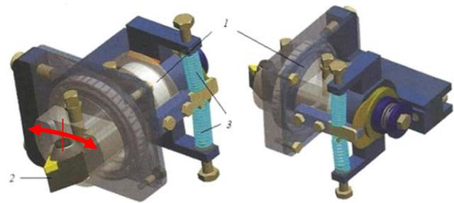
Figure 2. The virtual 3D CAD model of fixture with movable turning tool – design 1 (1 – roller bearings, 2 – turning tool, 3 – springs)
