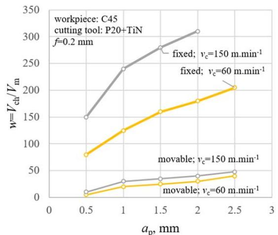
Figure 5. Experimental dependence of chip volume coefficient  $w$
