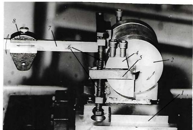
Figure 3. Fixture with movable turning tool – design 2; 1 – stand, 2 – pin with movable face disc, 3 – roller bearings, 4 – clamp, 5 – turning tool, 6 – springs, 7 – rod, 8 – movable weights balance
