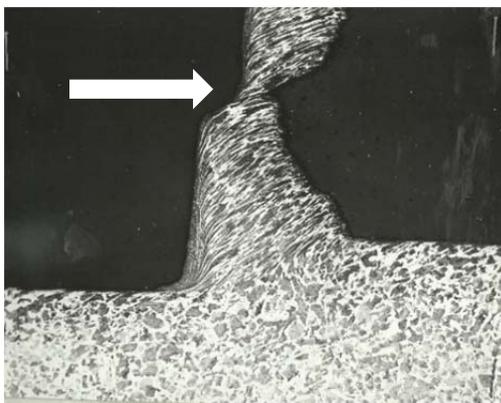
Figure 6. Metallographic cut of the chip of reduced thickness due to oscillation
