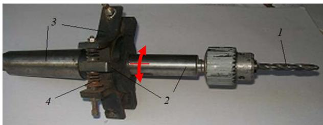
Figure 7. Fixture with movably mounted drill (1 – drill, 2 – shaft, 3 – fixture, 4 – springs)
