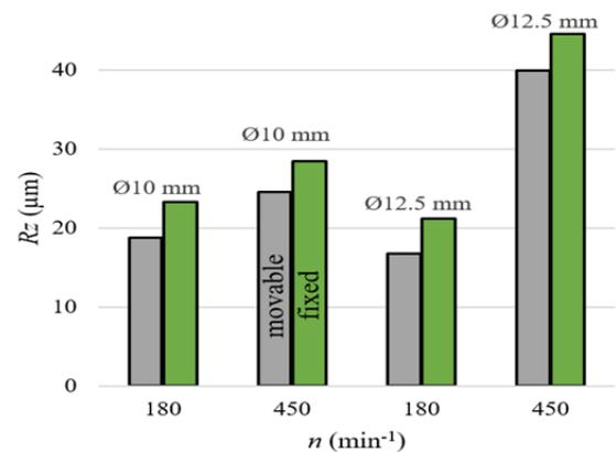
Figure 8. Maximum profile height  $R_z$ ; material of drill: HS-18-01, workpiece material: Fe37B1FU
