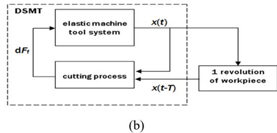
Figure 1. (a) Scheme of cutting tool within the machine-tool system; 1 – tool, 2 – workpiece, 3 – stiffness, 4 – damping,  $F_f$ ,  $F_p$ ,  $F_c$  is axial, radial, and tangential force, respectively, (b) dynamic system of machine tool (DSMT), cutting process (CP)
