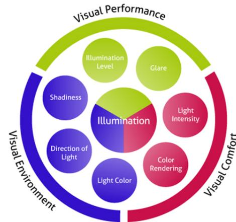
Figure 2. Illumination parameters in the working environment [6]
