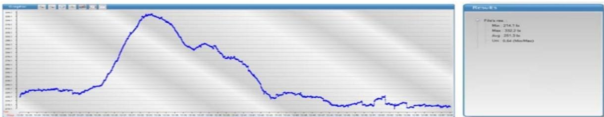
Figure 9. The intensity of illumination of the assessed workplace in time dependence (left) and a summary of obtained values (right) - Software LLX200
