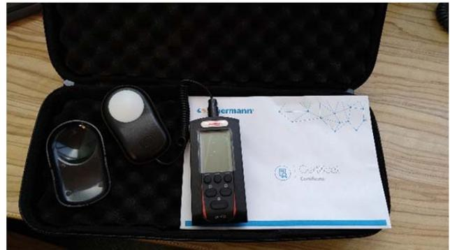
Figure 4. Digital lux meter KIMO LX200
