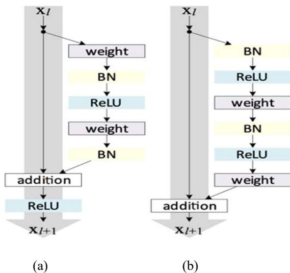
Figure 6. Architecture ResNetV1(a) and ResNetV2 (b) [16]
