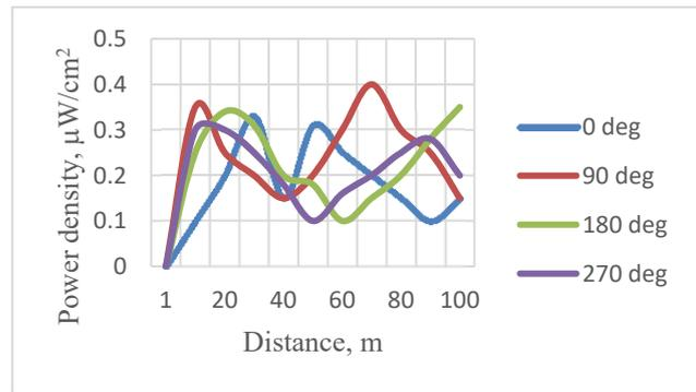
Figure 6. Distribution of the electromagnetic field power flux density at a height of 2 m from the ground in the direction of 0°, 90°, 180° and 270°
