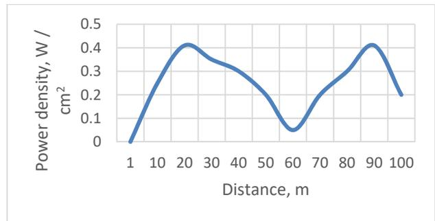
Figure 3. Distribution of the power flux density at a height of 2 m from the ground
