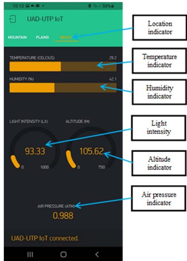
Figure 5. Indicator monitoring at the interface
