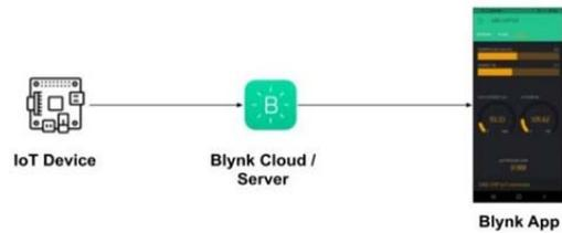
Figure 1. IoT-based smart weather system architecture
