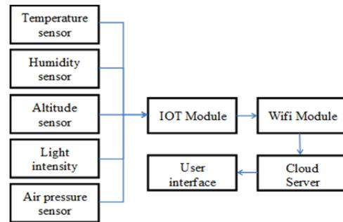
Figure 2. Block diagram of the IoT-based smart weather system
