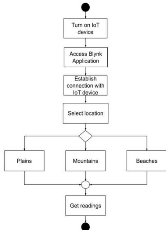
Figure 6. IoT-based smart weather system flowchart
