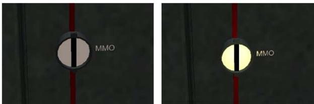
Figure 5. Discrepancy switch with light source switched off and on
