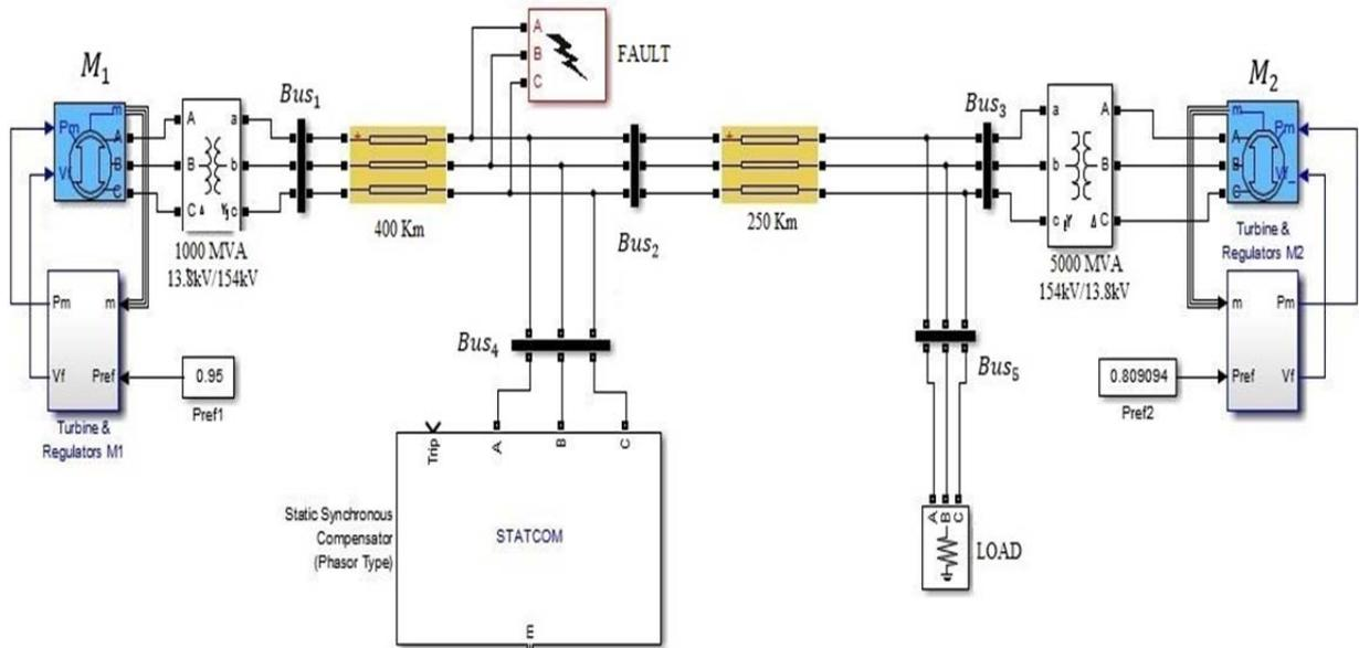
Figure 9. STATCOM system block diagram in case of asymmetrical and symmetrical fault [23]
