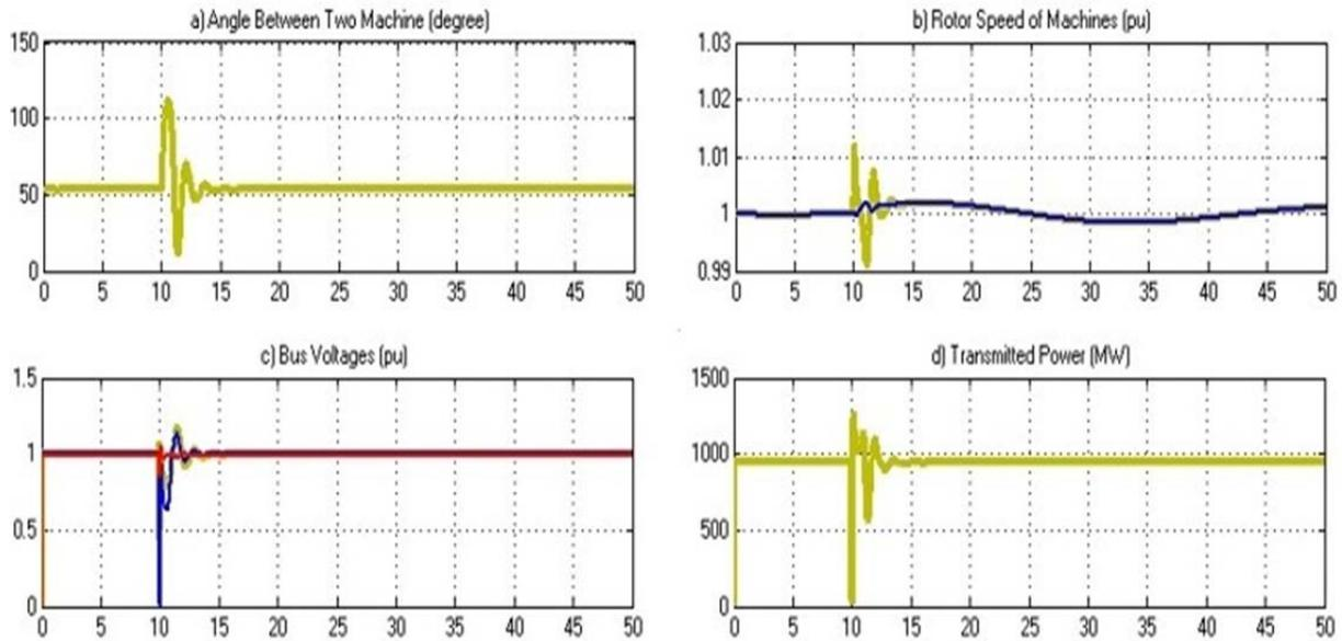
Figure 11. Effect of STATCOM on the system in case of symmetrical fault a) angle difference of generators b) rotor speeds of generators c) bus voltages d) power transmitted in the system
