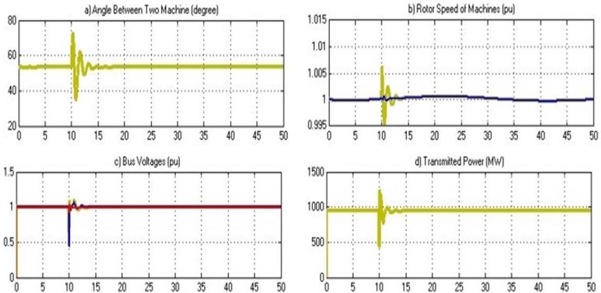
Figure 10. Effect of STATCOM on the system in case of asymmetric error a) angle difference of generators b) rotor speeds of generators c) bus voltages d) power transmitted in the system
