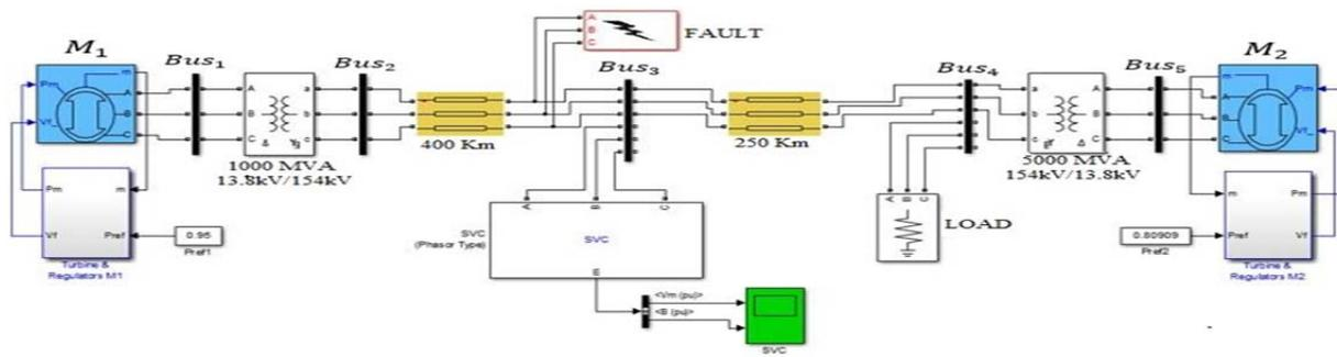
Figure 6. System block diagram with SVC during asymmetric and symmetric fault
