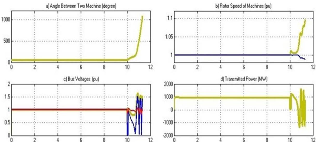
Figure 8. Effect of SVC on the system in case of symmetrical fault a) angle difference of generators b) rotor speeds of generators c) bus voltages d) power transmitted in the system
