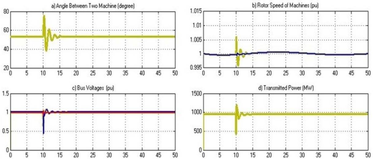
Figure 7. Effect of SVC on the system in case of asymmetric fault a) angle difference of generators b) rotor speeds of generators c) bus voltages d) power transmitted in the system
