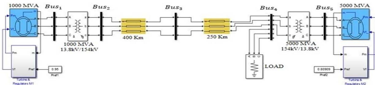
Figure 5. Simulink model of designed system [23]
