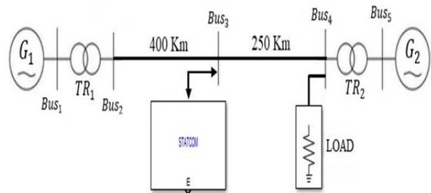
Figure 4. Two machine system with STATCOM
