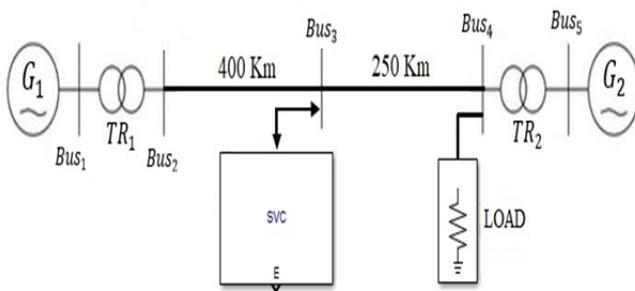
Figure 3. Two machine system with SVC
