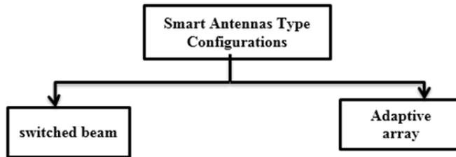
Figure 2. Type of Configurations Smart Antennas [14]
