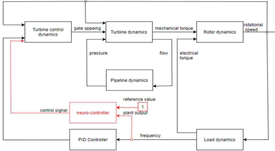
Figure 3. Block diagram of a hydropower plant [2] (amended by authors)
