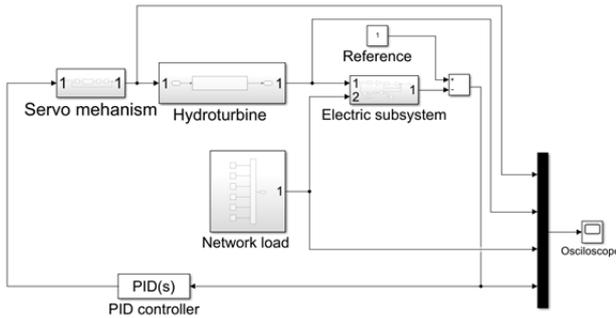
Figure 4. Simulink model configuration for PID models [2]
