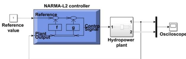
Figure 5. Simulink model configuration for NARMA-L2
