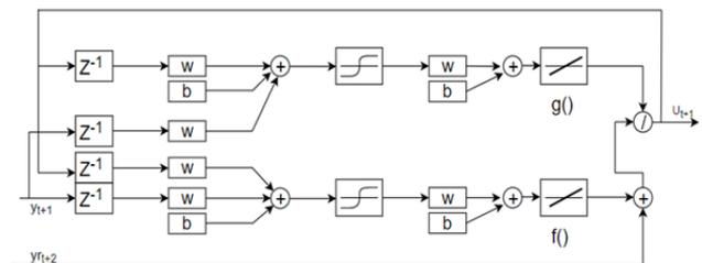
Figure 2. NARMA-L2 neuro-controller structure [13]
