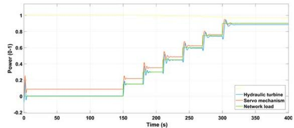
Figure 8. Response of a non-linear model of a turbine tracking the input signal using NARMA-L2
