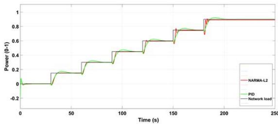
Figure 7. Comparison of the responses given by PID controller and neuro-controller
