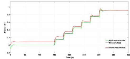
Figure 9. Response of a non-linear model of a turbine tracking the input signal using gain scheduling PID [2]
