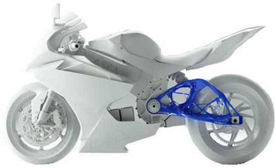
*Figure 1. Swivel arm developed by generative design technology by Lightning Motorcycles*
