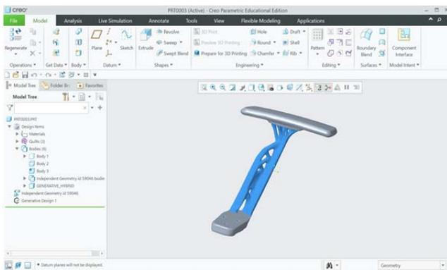
Figure 7. Dividing the model into required parts with the Multibody Design function
