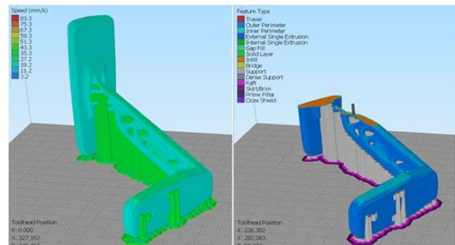
Figure 8. Simulation of the spatial printing of a model used for editing with generative design tools
