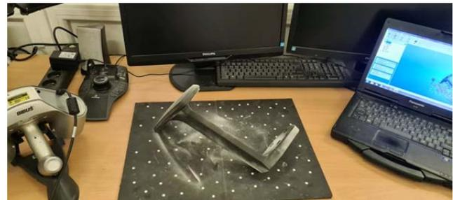
Figure 4. The process of scanning the chair backrest for CAD model creation
