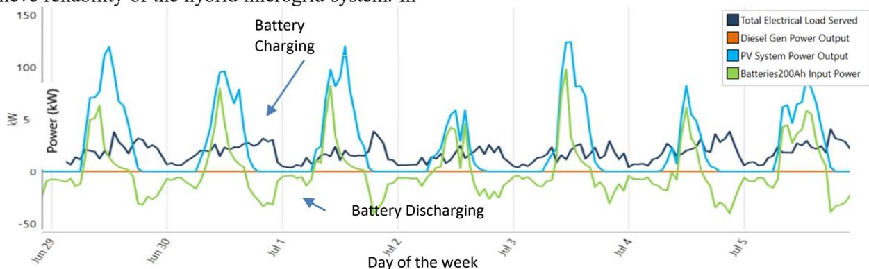
Figure 3. Power management for Lagundri microgrid
