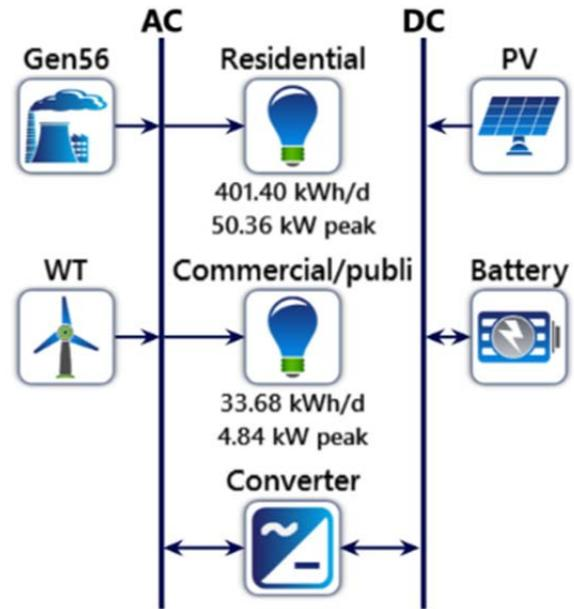
Figure 2. Proposed microgrid system components
