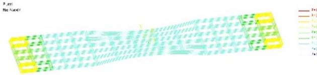
Figure 7. FEM model with mapped mesh control and polynomial order of the mesh
