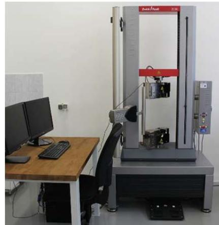
Figure 3. Tensile testing device for measuring the tensile strength of carousels
