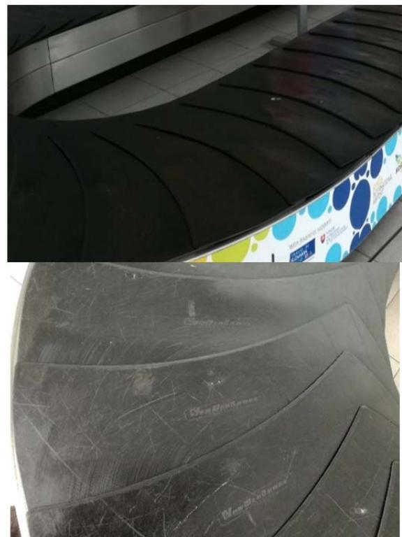
Figure 1. Damage to rubber carousels during the baggage conveyance at the airport
