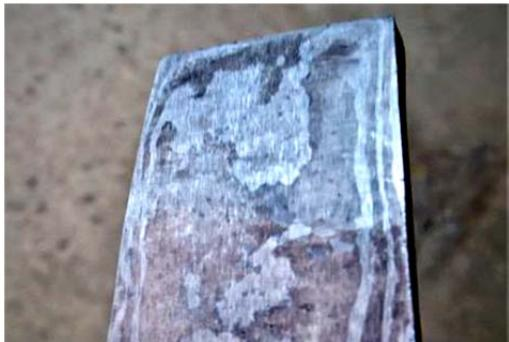
Figure 5. 20-layers damask made
