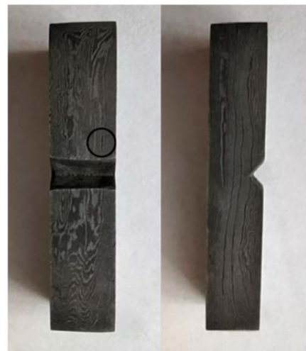
Figure 7. Sample for Charpy impact test (defect on the surface, outside of notch) / layers of test material
