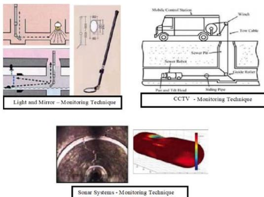
Figure 1. Sewer Inspection Technologies
