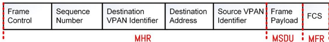
Figure 2. The IEEE 802.15.7 MAC frame structure [11], containing frame control, sequence number, address information and security-related information, frame payload, and frame check sequence (FCS)
