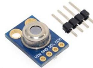
Figure 2. Non-contact temperature sensor
