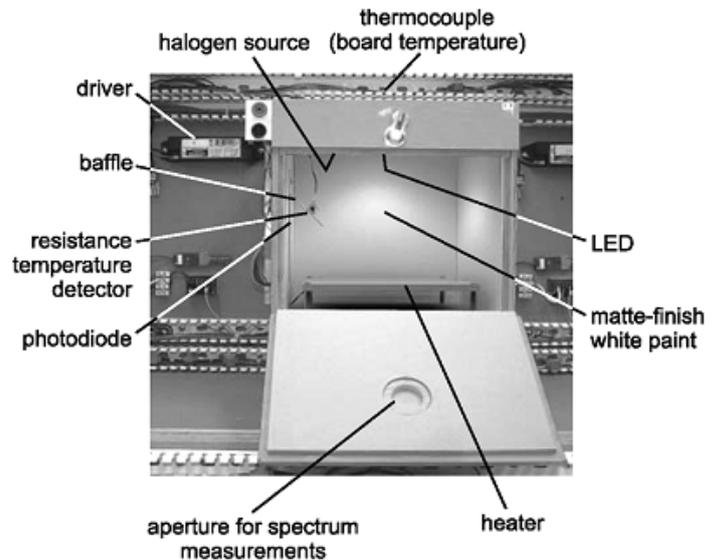
Figure 2. Placement of the elements inside the test chambers (as developed by the LRC)<sup>6</sup>
