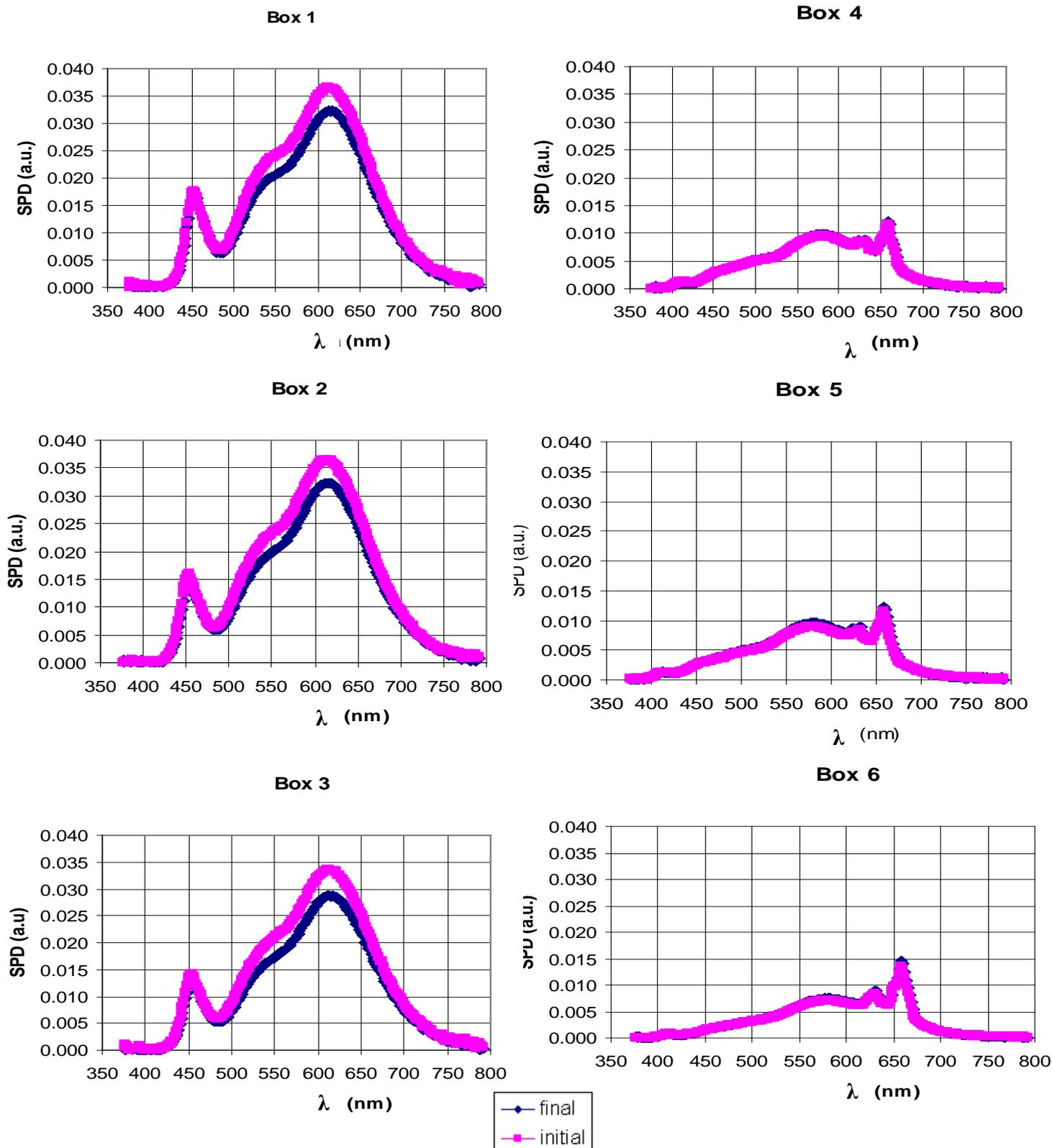
Figure 3. Initial and final SPD of the first (Box 1,2,3) and second group (Box 4,5,6) of LED
