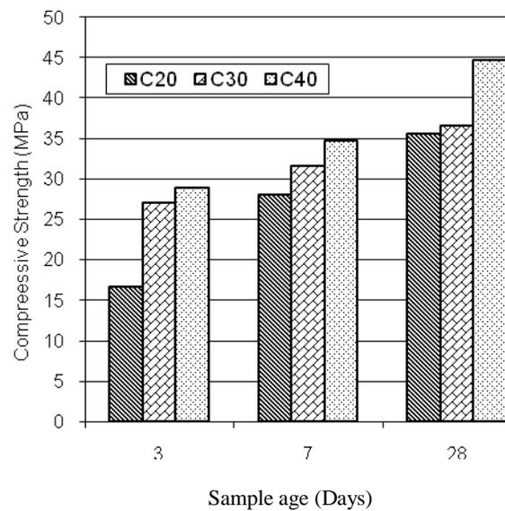
Figure 3. Compressive strength of concrete samples (Dmax: 16 mm).
