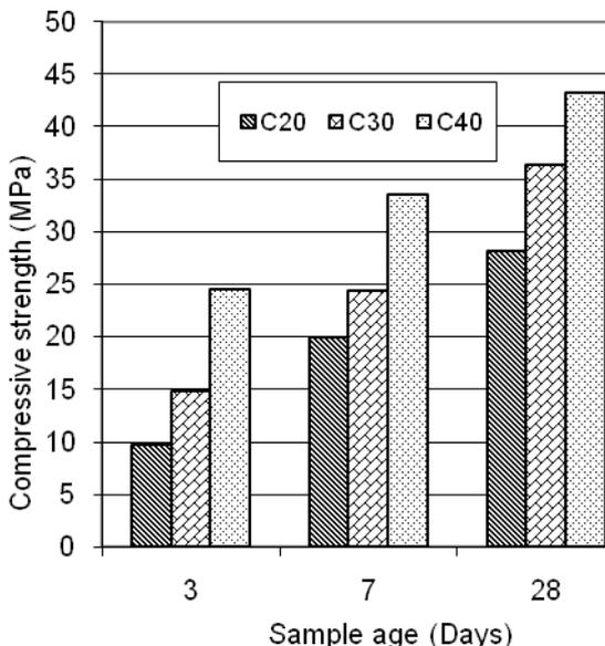
Figure 2. Compressive strength of concrete samples (Dmax: 31.5 mm).
