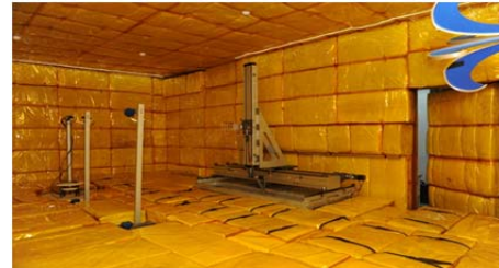
Figure 1. AEC with measurement equipment
