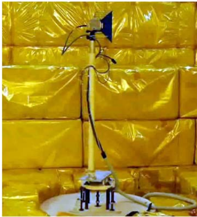
Figure 3. Antenna under test mounted on RAP
