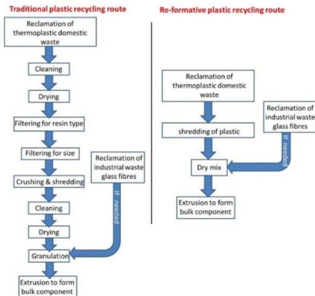
Figure 3. The schematic of the traditional plastic recycling process and the novel re-formative process
