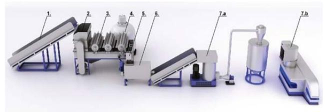
Figure 4. where: 1 - belt conveyor; 2 - crusher; 3 - sedimentary bath with a sieve; 4 - water filtration with chemical treatment; 5 - drainage screw; 6 - auger for squeezing; 7a - agglomerator + silo; 7b is a line of subsequent granulation
