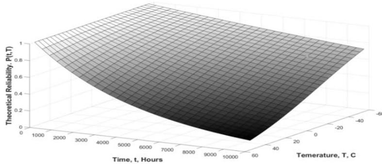
Figure 7. UAV communication unit reliability graph
