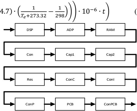
Figure 6. UAV communication unit reliability scheme
