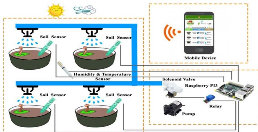
Figure 2. The infrastructure design of the vermiculture smart farming kit
