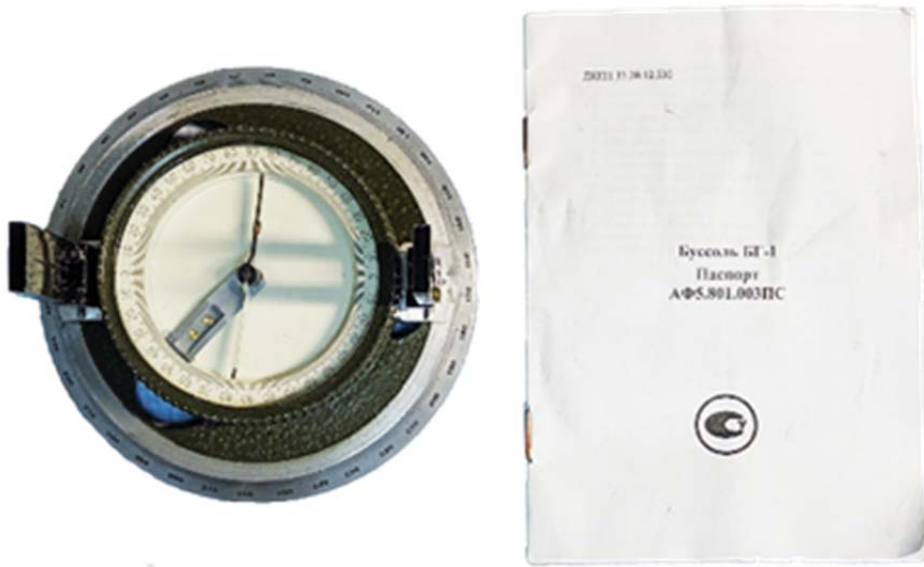
Figure 9. Reference compass used during field testing
