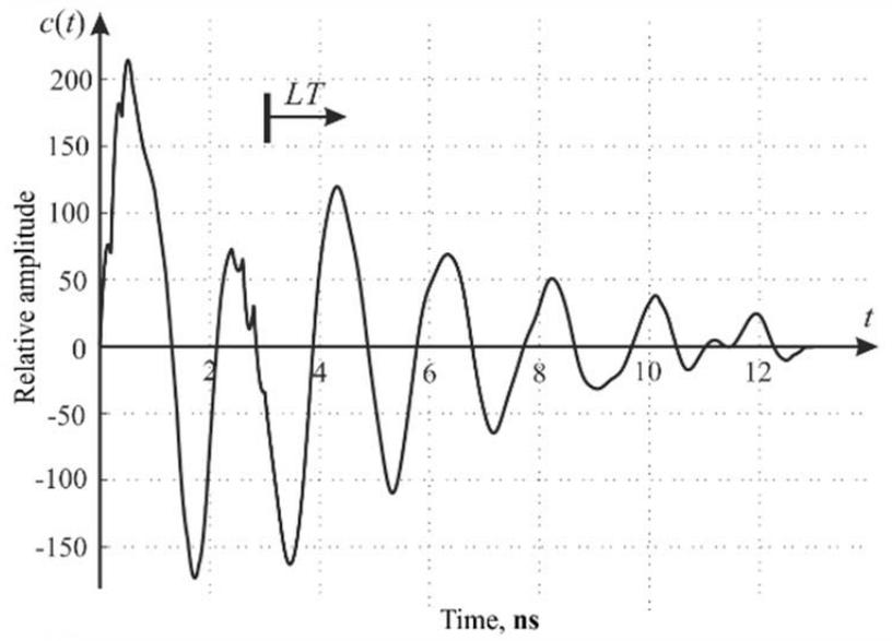
Figure 3. Cross convolution of F-18 response with the E-pulse fitted to B-707 pole set
