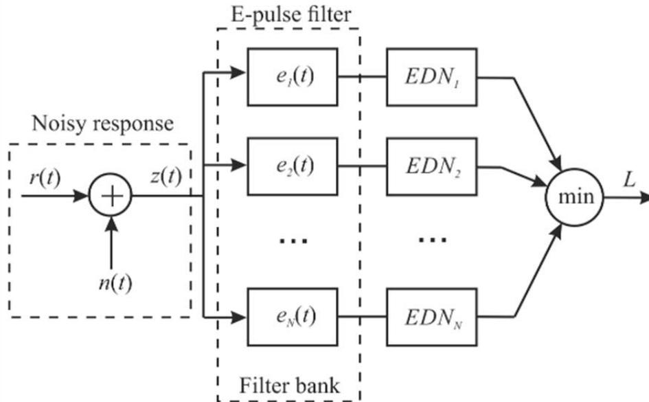
Figure 5. The structural scheme of the target discrimination system
