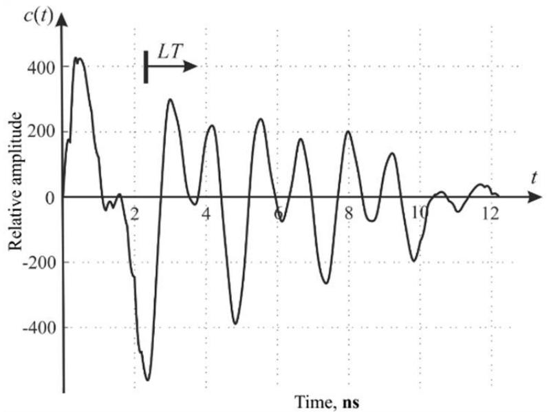
Figure 4. Cross convolution of B-707 response with the E-pulse fitted to F-18 pole set
