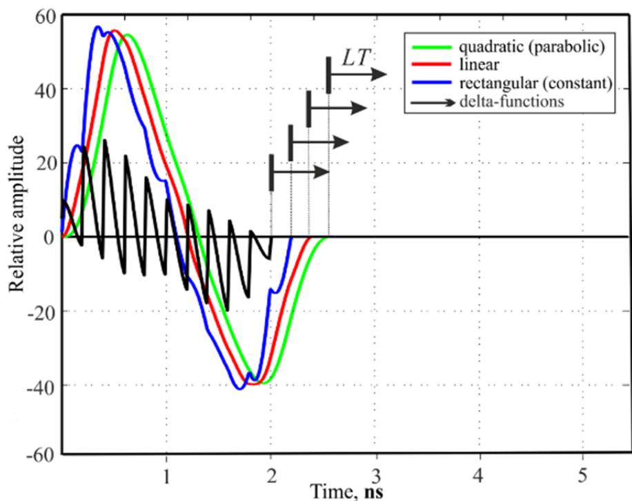
Figure 2. The convolution of F 18 response with the E-pulses fitted to F 18 poles
