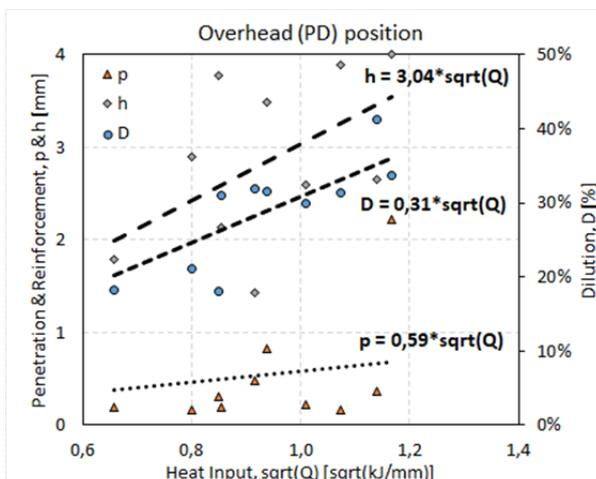
Figure 6. Penetration, reinforcement and dilution vs. heat input for overhead (PD) position
