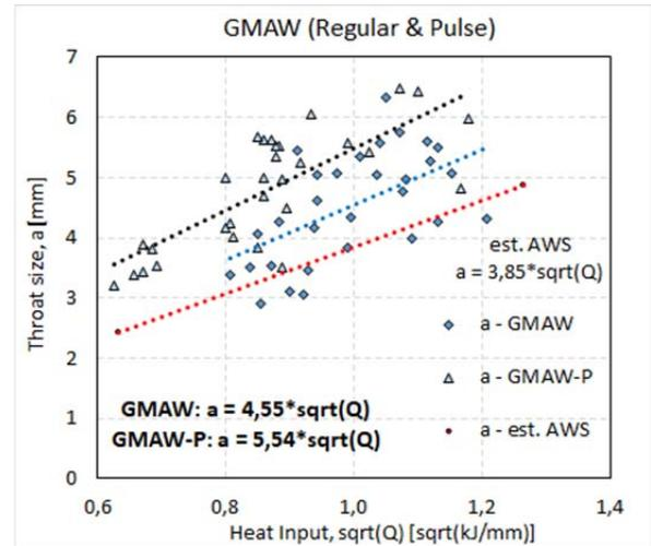
Figure 4. Throat size of fillet weld vs. heat input for GMAW and pulsed GMAW
