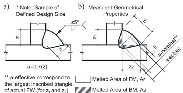
Figure 1. Geometrical properties of Fillet Welds
