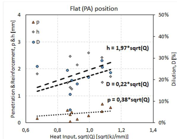
Figure 5. Penetration, reinforcement and dilution vs. heat input for flat position
